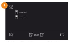
Select the panel from which you want to display the image. In case that the desired choice is a camera image, press to see the list of cameras.
